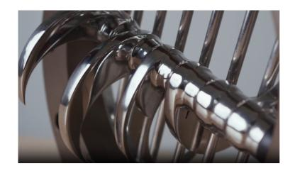
The lump-breaker is a tool designed to simplify the handling of materials that tend to form lumps or aggregates.
