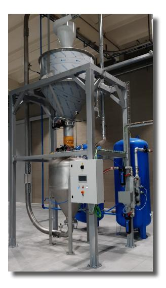
The **pressure vessels of the TPA line** are designed for handling a wide range of materials and blends of different products. They are also recommended for applications over long distances and with large rates; also able to ensure the integrity of the material and limit wear on the pipes.
