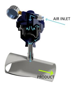
The booster is a device designed to convey bulk materials evenly through a dense-phase pneumatic conveying line.
